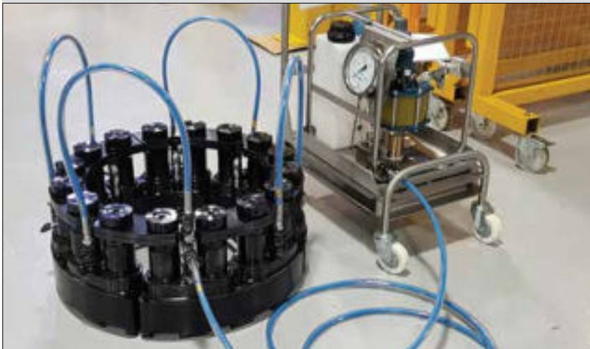
▲ Multi-Stud Tensioning Set-Up.
