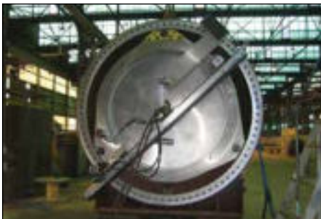
▼ Wind tower machining with WP4600.
