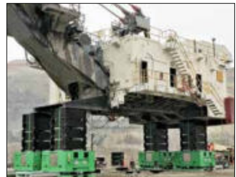
▼ Undocking an 1500-ton Electric Rope Shovel in a Copper Mine with a JS500 Jack-Up System for bearing inspection and maintenance.
