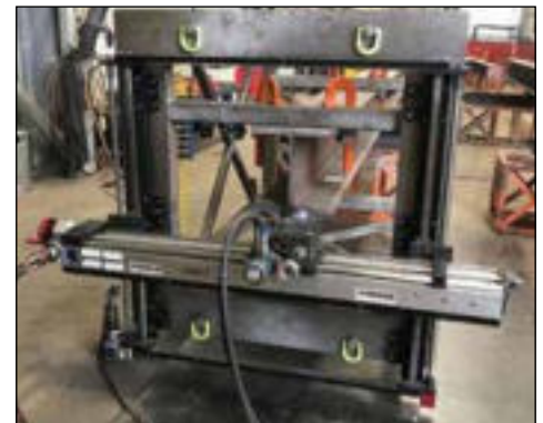
I-Beam end face milling with a GMRF1000.
