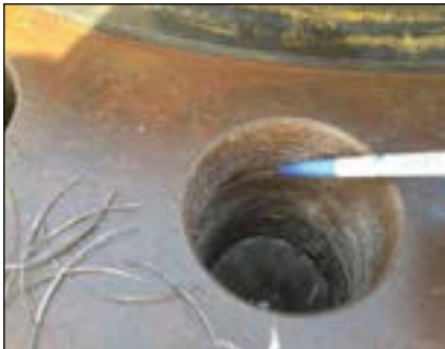
▲ A typical thread before refurbishment
