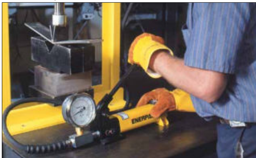
▼ A GP10S gauge is used on this press to check the hydraulic pressure required to bend a steel plate.
