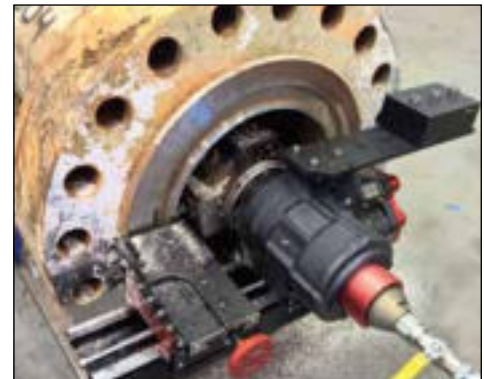
▼ MM8601 machine to ensure flange joint integrity.
