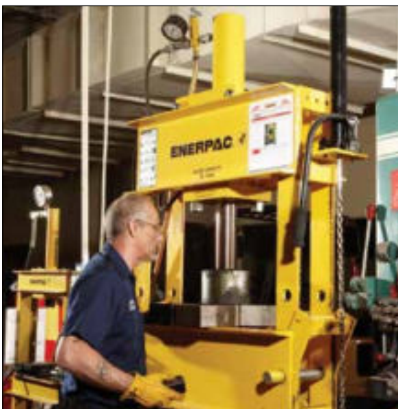
◀ An Enerpac H-Frame press quickly removes the shaft from this assembly.
