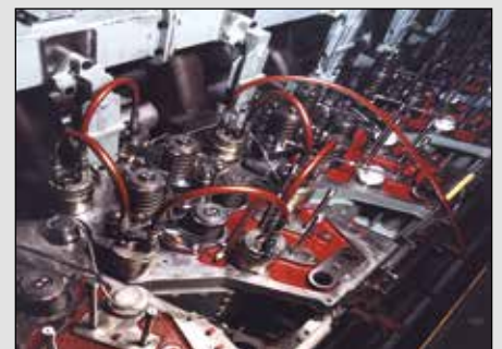
▲ Hydraulic nuts on a diesel engine.
