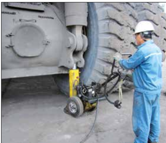
◀ Enerpac POW'R-RISER® used in mining operations to lift heavy equipment.
