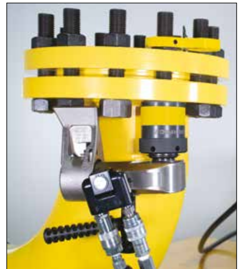
▲ Hands-free torque wrench system: STLLS-model with S-Series torque wrench. The square drive of the wrench can easily be exchanged by the Safe T™ Torque Lock model.
