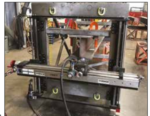
I-Beam end face milling with a GMRF1000. ▶
