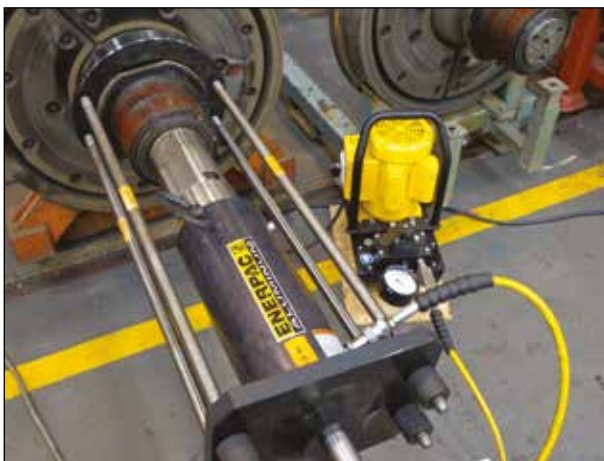
◀ Rail wheel pulling using RACH aluminium cylinder powered by ZE-Series pump.
