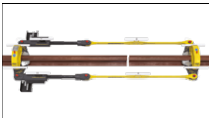
▲ Modular 70 ton stressor and holds the rail in neutral length during the welding process.
