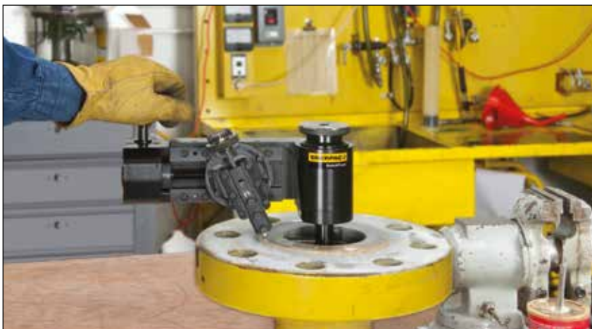
▼ The Enerpac FF120 used to face a pipe flange.
