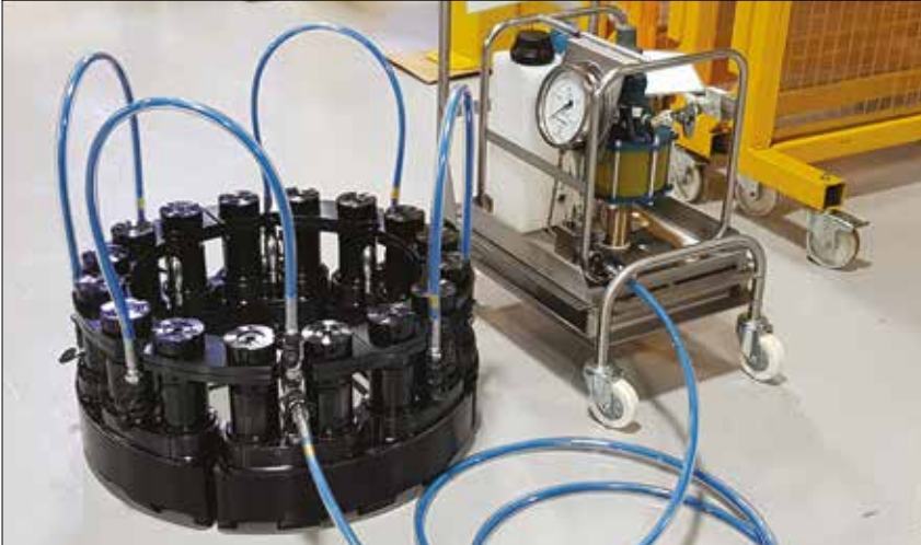
▲ Multi Stud Tensioning Set-Up.
