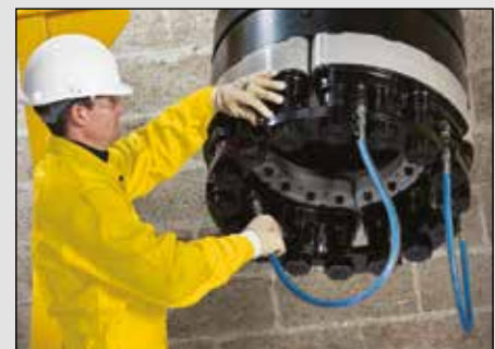
▲ Multi Stud Tensioning application.
