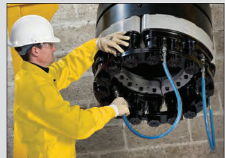
▲ Multi-Stud Tensioning application.
